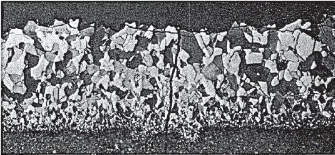
Figure 1: Two different CVD ZrC coatings (~90 \mu m thick) on a graphite composite substrate showing columnar microstructure (top) and an equiaxed microstructure structure (bottom). From [16]
