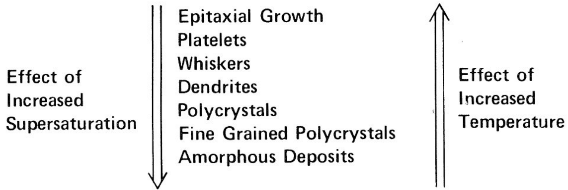
Figure 2: Effect of supersaturation and temperature on the structure of vapor deposited materials. After [13]
